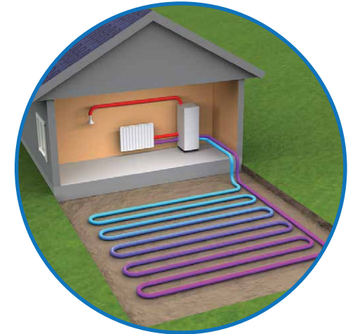
Ground Source Heat Pump diagram (Source: Incognito Heat Company)
